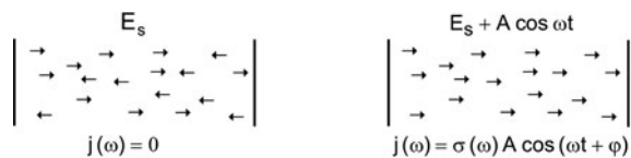
Fig. 32.10 Bloch oscillations of miniband electrons under the action of a static field (left), and of both a static and a high frequency field (right)
