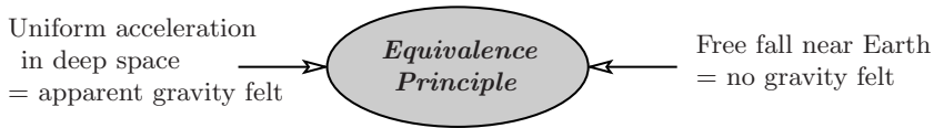
Fig. 12.1. The Equivalence Principle has two sides. One is that uniform acceleration far from any source of real gravity will be felt as an apparent gravity, “apparent” because the pseudo-potential is constant. The other side of the principle says that during free fall in a real gravity field, no gravity at all will be felt; in a small region, our frame will be inertial.
