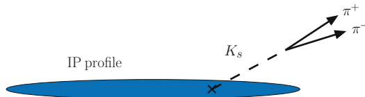
Fig. 6.2 Figure illustrating K_S vertexing. The B^0 - \bar{B}^0 system is boosted in the z -direction, leading to an elongated “IP profile,” where IP stands for Interaction Point. Although the decay lifetime of K_S from B decay is not optimal for the silicon vertex detector, intersecting the K_S momentum with the IP profile gives some information of the B meson decay vertex
