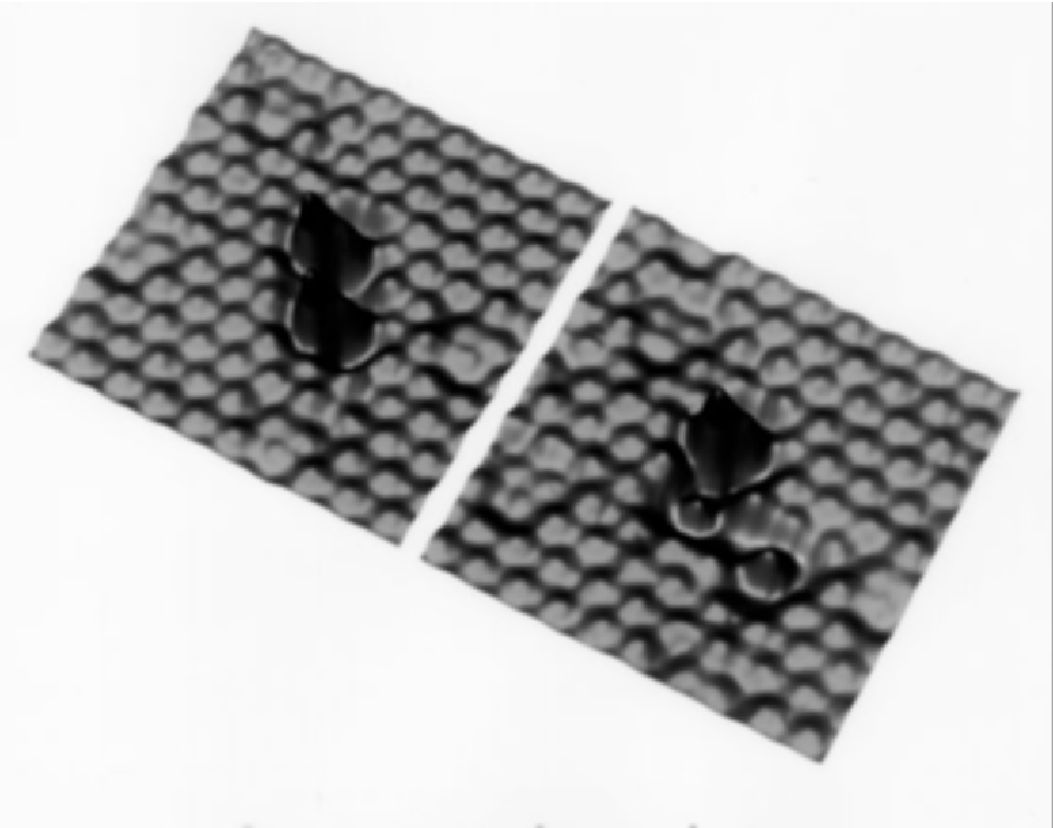
FIGURE 21.1 Upper left: Two O_2 molecules are revealed by the scan of an STM; lower right: Scan of the same two molecules after a voltage pulse has been delivered to one. The scan shows that the O_2 molecule has been separated into two O atoms. Picture courtesy of Wilson Ho, Department of Physics and Astronomy, University of California, Irvine.
