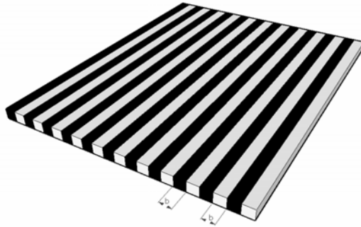
FIGURE 10.28 A diffraction grating made of alternating strips of transparent and opaque material (Problem 18).
