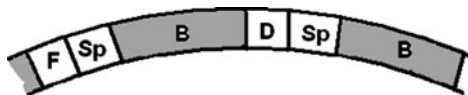
Fig. 11.7 A FODO half-cell F – focusing, D – defocusing quadrupole, B – bending magnets and Sp – Spool pieces
