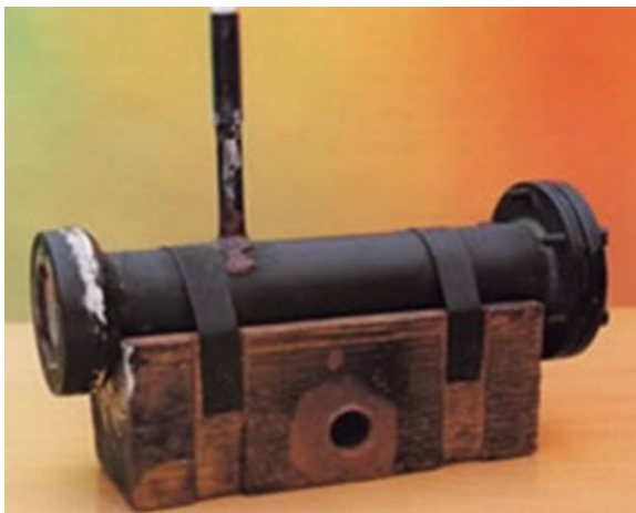
Fig. 3.4 James Chadwick's neutron experimental apparatus. Image 10313943, Science Museum, Science and Society Picture Library
