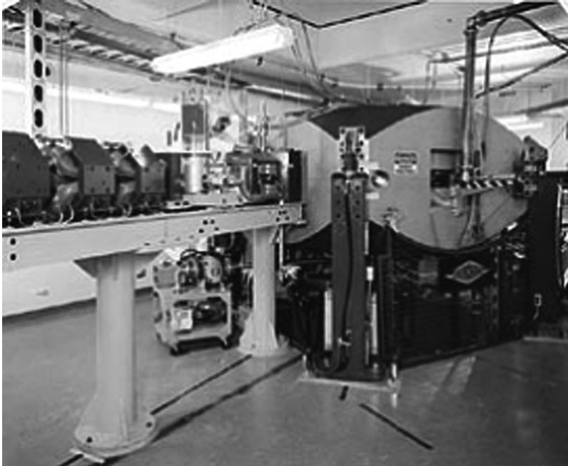
Fig. 5.10 An Advanced Cyclotron Systems 30-MeV variable energy, 1.2-mA negative ion cyclotron for isotope production (Courtesy: Advanced Cyclotron Systems, Richmond, B.C., Canada)
