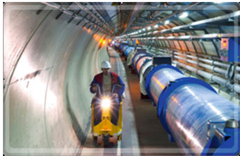
Fig. 13.3 The double beam tube (2 in 1) superconducting dipole bending magnet (Courtesy, CERN, European Organization for Nuclear Research, Geneva, Switzerland)
