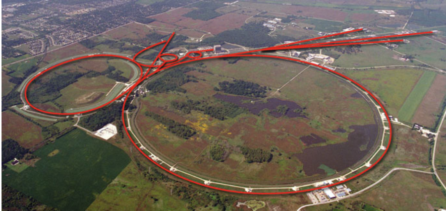
Fig. 8.10 Aerial picture showing the Tevatron at Batavia, Illinois, USA (Illustrated with red line). The larger ring is the Tevatron and the smaller one the Main Injector (Courtesy: Fermi National Accelerator Laboratory, IL, USA)
