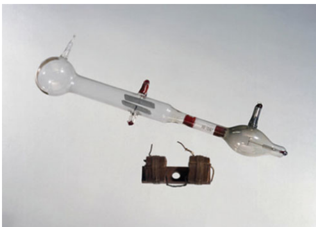
Fig. 2.1 J.J. Thomson's Cathode Ray Tube with deflecting electrodes and Helmholtz coils. Image No. 10324719 © Science Museum/Science & Society Picture Library
