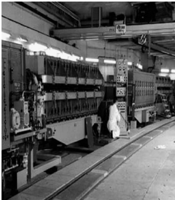
Fig. 7.7 CERN's 28 GeV Alternating Gradient Proton Synchrotron. The alternating gradient can be seen as one C magnet with the open side facing out and the next facing in, as envisioned by Livingston. Courtesy: CERN, European Nuclear Research Organization, Image Reference : CERN-AC-5901157)
