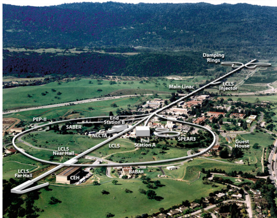
Fig. 9.9 2 mile long linear accelerator (the straight line heading to top right), at SLAC. Photographed in 2006. The figure also shows a circular machine PEP II in the foreground. The linear accelerator injected electrons and positrons into two rings in PEP II, which were then collided. (Courtesy: SLAC National Accelerator Laboratory)
