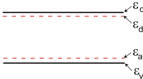
Fig. 7.3. Impurity levels in semiconductors doped with N_d donors and N_a acceptors per unit volume
