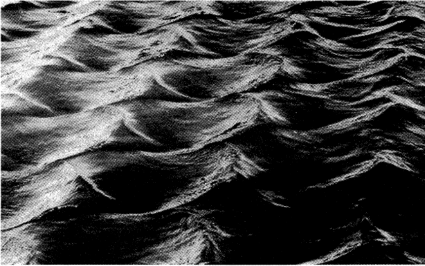
Fig. 8.6. Three-dimensional wavestructures [illustration courtesy of Ming-Yang-Su and M. van Dyke, Ed. An Album of Fluid Motion (The Parabolic Press, Stanford 1982) Fig. 194]
