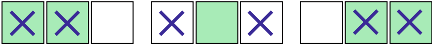
Fig. 4.17 Schematics showing three possible combinations of L1 triggers leading to an L2 trigger in the upper and lower rings of antennas. Blue crosses indicate L1 triggers, green shaded regions indicate L2 triggers. Note that only three antennas (from a ring of 16) are shown, all other antennas are assumed to have not been triggered
