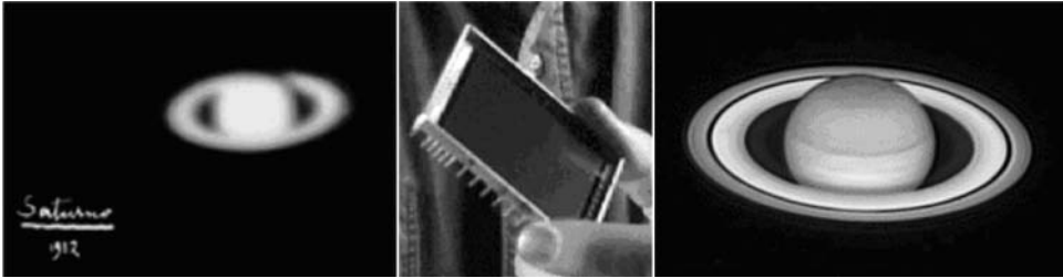
FIGURE 5.2. An example of the advantages that can be achieved by using a CCD (centre): (left) an image of Saturn obtained in 1912 from the Collurania Observatory (Teramo, Italy) (right) an image obtained with a CCD on a modern commercial telescope.
