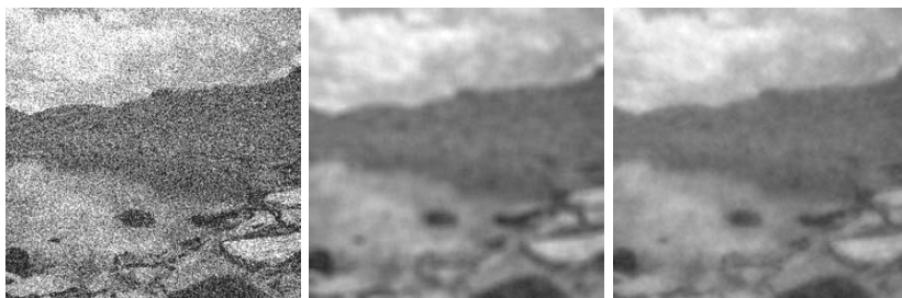
Fig. 6.7 Example of the trade-off between different parameters. Left: Original image, 256 \times 256 pixels, with additive Gaussian noise, standard deviation \sigma = 50 . Middle: Denoising with E_D , radius r_D = 5 . Right: Denoising with E_C , \alpha = 0.424 . Source: [47]
