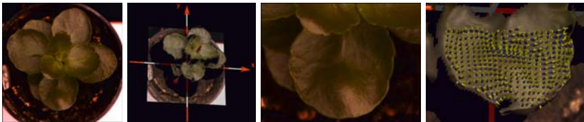
Fig. 7.18 Reconstruction of plant using 49 camera positions. From left to right: central image of input sequence, rendered depth estimates, close-up view on leaf and estimated depth with surface slopes
