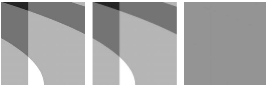
Fig. 3.5 From left to right: initial geometric image f , \tilde{u} , \tilde{v} + 150 , computed with Db3 in the translation invariant setting, \alpha = 0.5 , \gamma = 0.01
