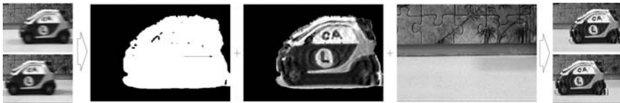
Fig. 4.12 From two real blurred frames ( left ), we automatically and simultaneously estimate the motion region, the motion vector, and the image intensity of the foreground ( middle ). Based on this and the background intensity we reconstruct the two frames ( right )
