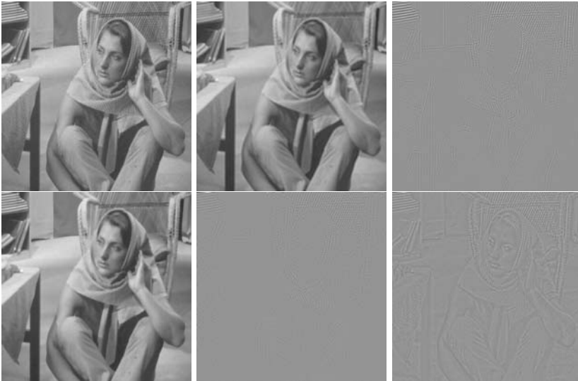
Fig. 3.8 Top from left to right: initial woman image f , \tilde{u} and \tilde{v} + 150 , computed with Db10 (Method C), \alpha = 0.5 , \gamma = 0.002 ; bottom from left to right: u and v obtained by the Vese–Osher TV model and the v component obtained by the Vese–Solé–Osher H^{-1} model
