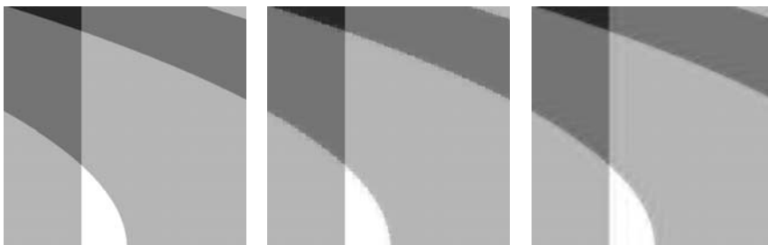
Fig. 3.4 An initial geometric image f (left), and two versions of f (the middle decomposed with the Haar wavelet basis and the right with the Db3 basis) where the soft-shrinkage operator with shrinkage parameter \alpha = 0.5 was applied
