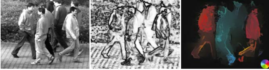
Fig. 4.11 Pedestrian video: frames from original sequence ( left ); phase field ( middle ); optical flow, color coded ( right )
