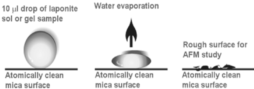
Figure 13. Sketch of sample preparation for AFM studies of rough deposited surfaces of laponite [13].
