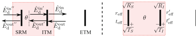
Fig. 2.14 Mapping from a three-mirror cavity to a two-mirror cavity by defining the effective transmissivities ( t_{\text{eff}} , t'_{\text{eff}} ) and reflectivities ( r_{\text{eff}} , r'_{\text{eff}} ) of the signal-recycling cavity
