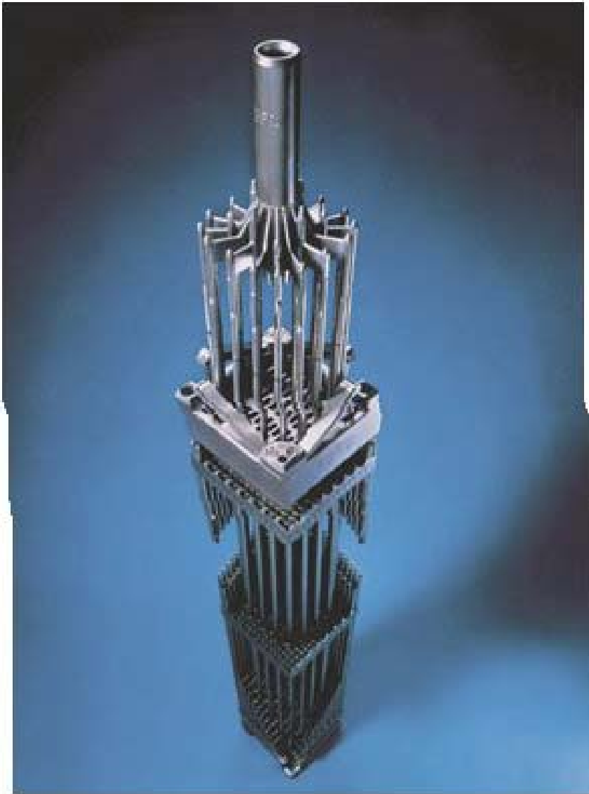
Fig. 6.9. Fuel element holder for a PWR reactor. The figure shows the control rods in place. When filled, the structure contains 264 zirconium tubes of length 4 m and diameter 9.5 mm containing pellets of \text{UO}_2 .
