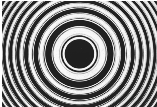
FIGURE 2.21 A Fabry–Perot ring pattern obtained using the green line of the mercury spectrum (from Cagnet, Francon, and Thierri, Atlas of Optical Phenomena , Springer-Verlag, Heidelberg, 1962).
