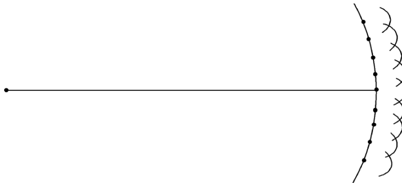
FIGURE 3.1 Schematic of wavefront construction using Huygens' Principle.
