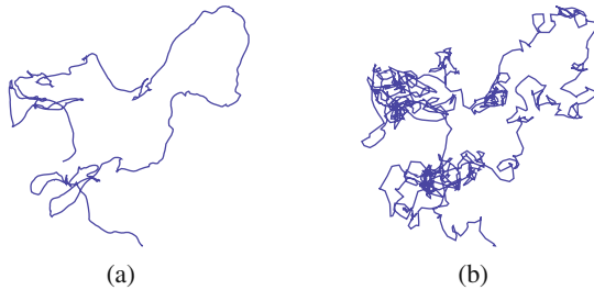
Fig. 1.2 Two-dimensional trajectories of a free Brownian particle. (a) A solution x(t) of (1.16), (b) A solution x(t) of (1.19). In (a) , the velocity of the Brownian particle ( \sim v_{th} ) is approximately maintained along the segment for \sim v_{th}(m/\gamma) . In (b) the trajectory shows fictive fine structures even below the length v_{th}(m/\gamma)
