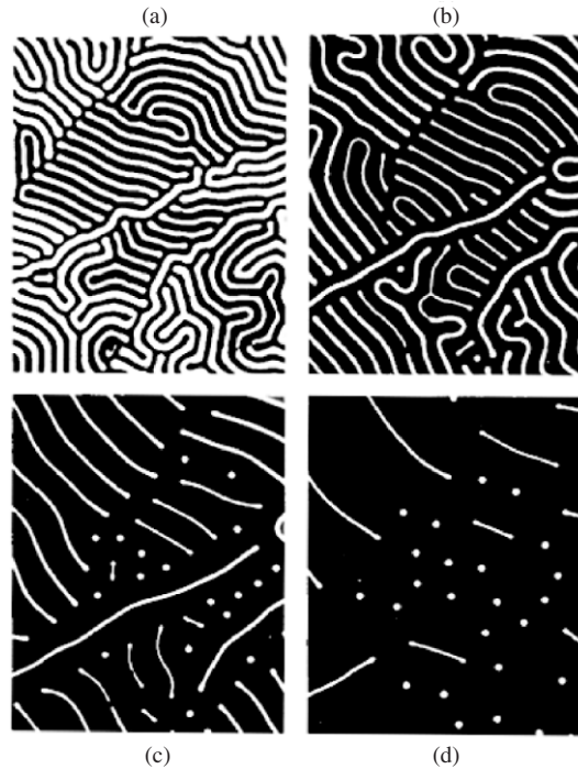
Fig. 9.10. Magnetic domains. A magnetic material is composed of a large number of magnetized regions called domains. The domains in a thin film (6 microns) of YGdTm are shown here. (a) Non-magnetic phase; (b, c, d) magnetization in an increasing magnetic field; magnetic bubbles are formed (A. H. Bobeck and E. Della Torre, in: Magnetic Bubbles , North Holland, 1975)
