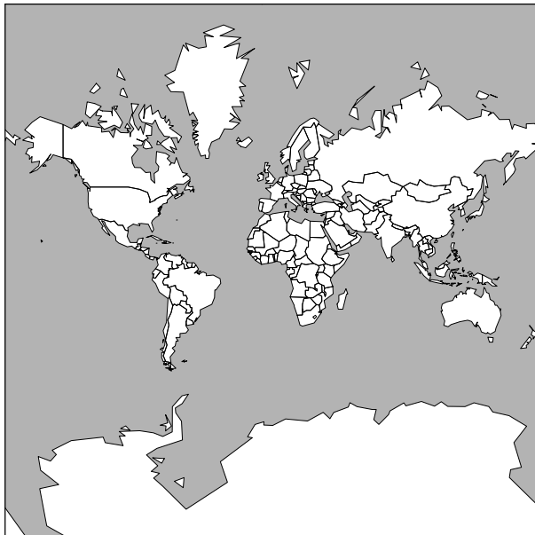
Fig. 1.10. A map of the world using the Mercator projection. Since the entire map would have infinite height, only the portion between 85^\circ\text{S} and 85^\circ\text{N} is shown here.
