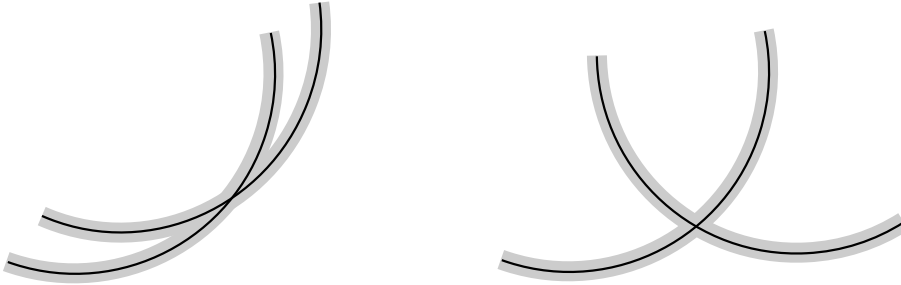
Fig. 1.2. A small angle of intersection at the left (loss of precision) and a large angle at the right.
