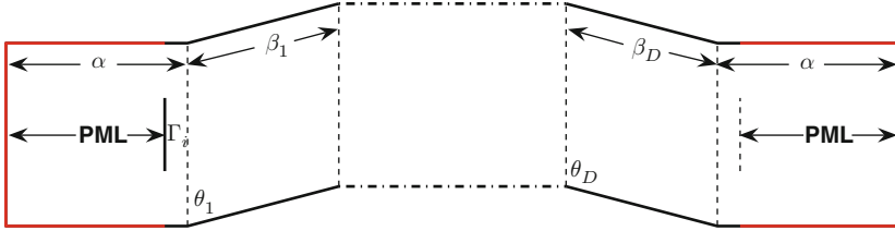
Fig. 4 A general domain decomposed into D + 2 subdomains
