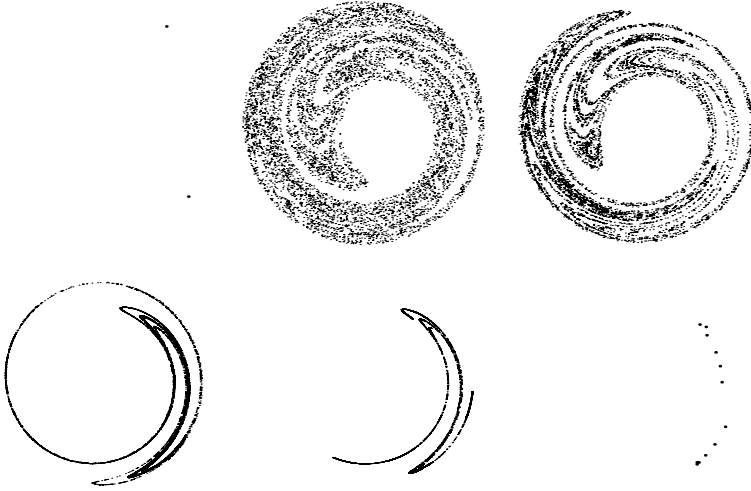
Figure 6.11: The figure depicts the attractor for the stroboscopic Poincaré map for the system \ddot{\theta} + \mu\dot{\theta} + \sin \theta = -1/10 + 2 \cos(2t) \sin \theta where, from left to right, \mu = 0.03, 0.0301, 0.1, 0.5, 0.56, and 0.65 .
