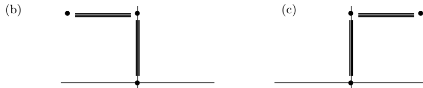
Figure 2.5 Difference stencils of the implicit discretizations (3.31)
