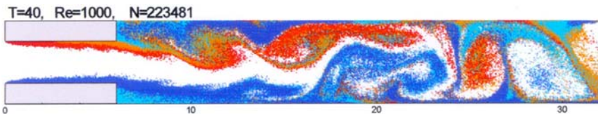
Figure 3.21. Cubic B-splines are used to solve the diffusion problem that arises in the study of vortex transport. This figure shows the formation of eddies in the flow of fluid as it moves through a small narrow chamber (Kudela [1999]).
