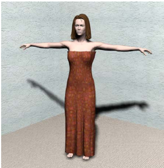
Figure 1.5. The animation of deformable objects using physically based modeling involves solving differential equations in which A-stability is an essential property of the numerical scheme. The example shown here uses backward Euler, and the trapezoidal method, to simulate the motion of clothing on a woman model (Hauth and Eitzmuß [2001]).
