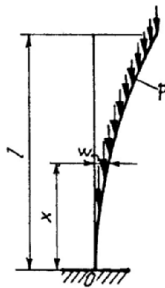
Figure 1. 56. Buckling of a cantilever bar acted upon by an axial uniformly distributed load
