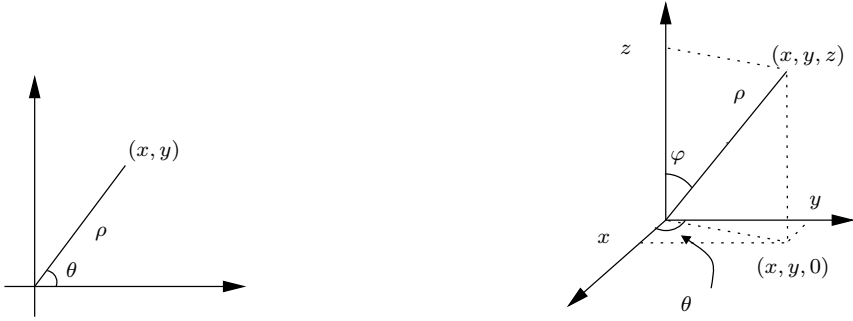
Figure 1.23. From the left: (i) Polar coordinates in \mathbb{R}^2 and (ii) Spherical coordinates in \mathbb{R}^3 .
