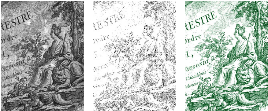
Fig. 1.2 Example: Picture of a 300-year-old globe. Left: The original image. Middle: The initial set consists of black pixels that are detected by global thresholds. Right: The binary result
