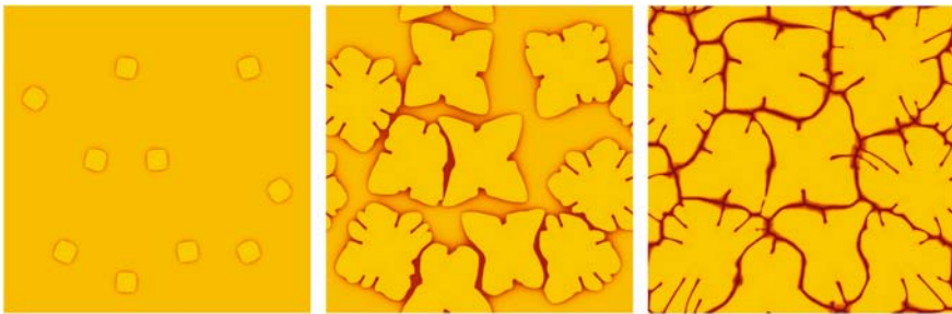
Fig. 4.17. Growth of dendritic NiCu grains into a 20 K undercooled melt illustrated by the Ni concentration (range: 0.41–0.62). The complete solidification (right image) is reached after further reducing the temperature by 15 K in a second step. (This figure is displayed in the text on page 143.)
