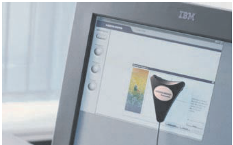
Figure 67 Calibration of a monitor for color-consistent soft proofs using the example of ViewOpen® from Heidelberg
