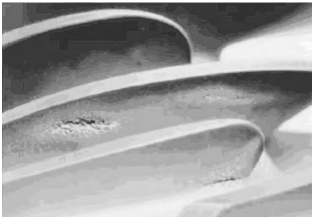
FIGURE 5.10 Typical blade damage due to cavitation of a mixed flow pump.
