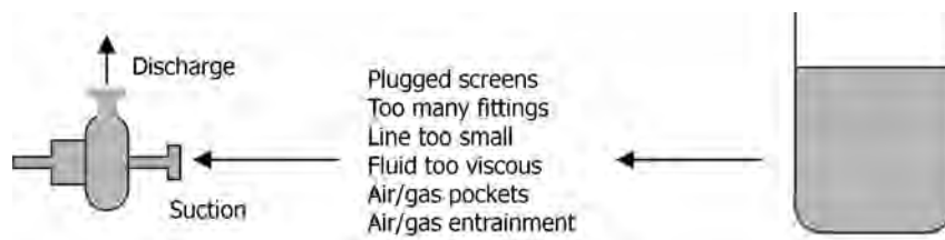
FIGURE 5.13 Pump suction side problems.
