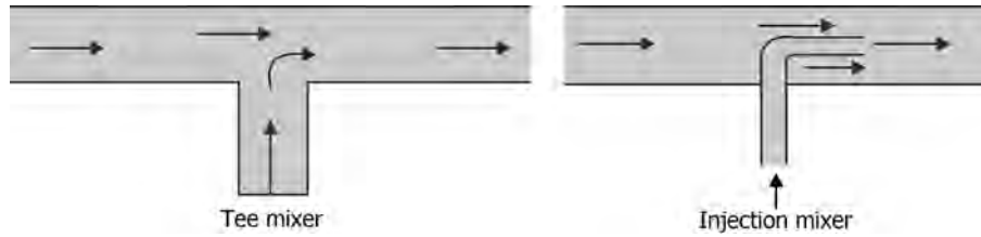
FIGURE 6.16 Tee and injection mixers.
