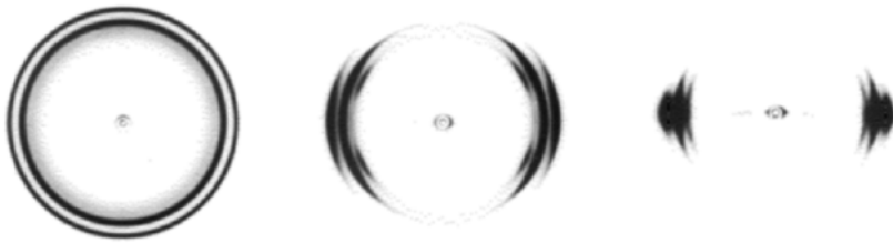
Fig. 10.17. X-ray scattering patterns of PE, as registered for the isotropic part ( left ), the center of the shoulder ( center ) and the neck ( right ) of a cold-drawn sample. The two reflections in the isotropic pattern are to be assigned to the 110-lattice and the 200-lattice planes of orthorhombic PE. The third reflection with a larger lattice plane spacing emerging in the textured patterns is due to a triclinic crystalline phase that forms during drawing [126]
