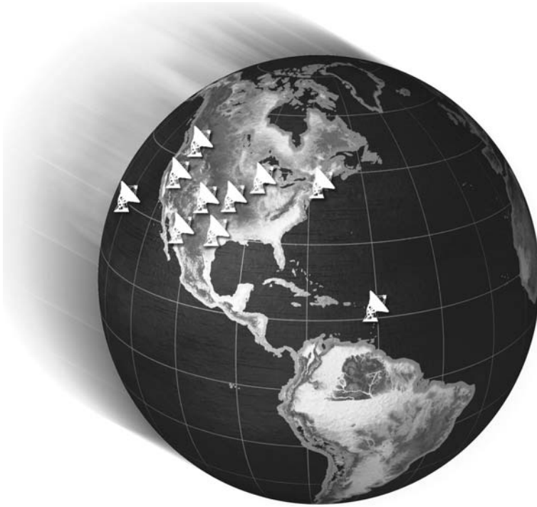
FIGURE 1.5. The location of the 10 dishes that make up the VLBA radio telescope of the National Radio Astronomy Observatory. Data from all the out stations are brought together at the central processing computer in Socorro, NM. (Image courtesy of NRAO/AUI.)
