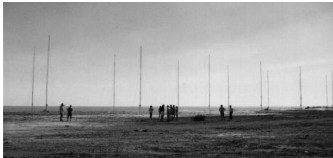
Fig. 2. Receive array of the SECAR HF surface wave radar
