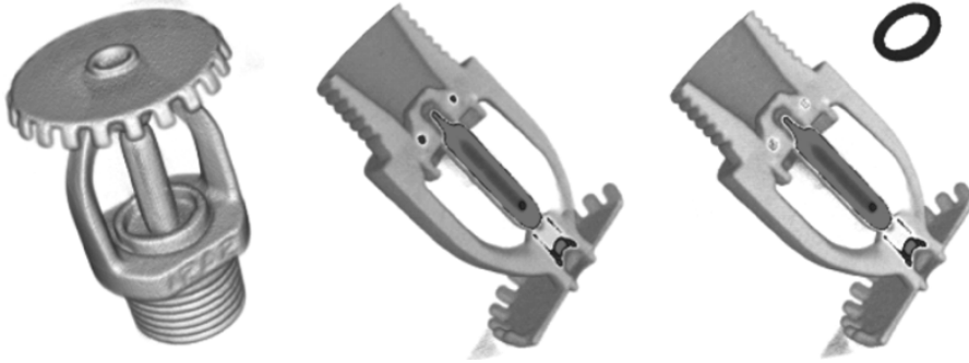
Fig. 15.7. Neutron tomography images of a sprinkler nozzle – outer surface, central slice, segmented O-ring. The object has a length of about 5 cm. The liquid in the glass capsule and the rubber ring gives especially high contrast for neutrons compared to the metallic structure
