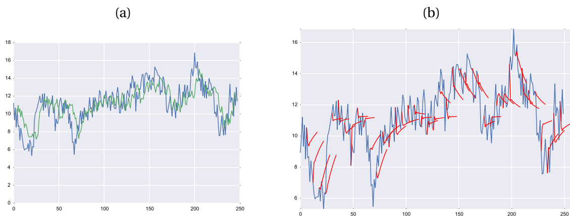
Figure 25.1: The left panel shows the forecast plot for h = 5 and the right panel shows a hedgehog plot with h = 10 where the skip parameter is set to 5.
