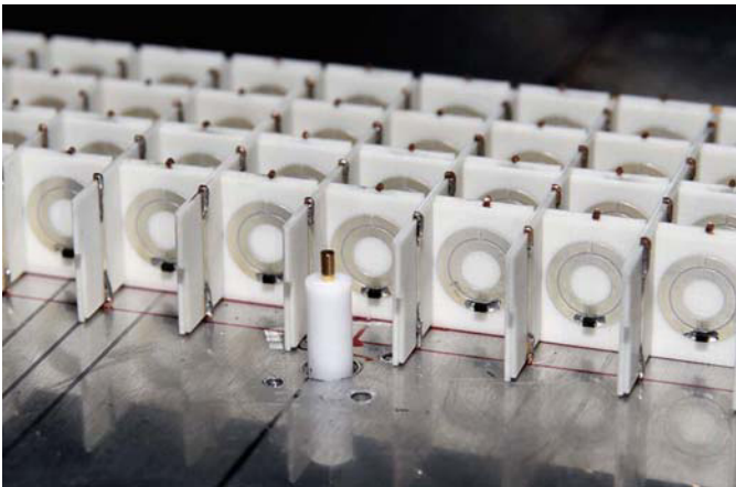
Fig. 14.3. Photograph of nonlinear metamaterial. Each SRR in metamaterial contains varactor diode (Skyworks SMV1405)
