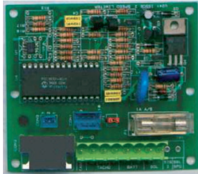
Fig. 8.36. The electronic control unit of the speed limiter using a PIC 8-bit micro-controller
