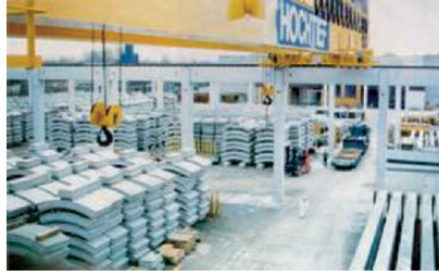
Fig. 8.60. The 64 ton crane of Hochtief Corp. uses fuzzy PLC based antisway positioning control (Video)
