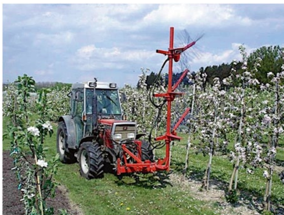
Fig. 4.6 Mechanical blossom thinning performer in an apple orchards in Germany. (Damerow and Blanke 2009)
