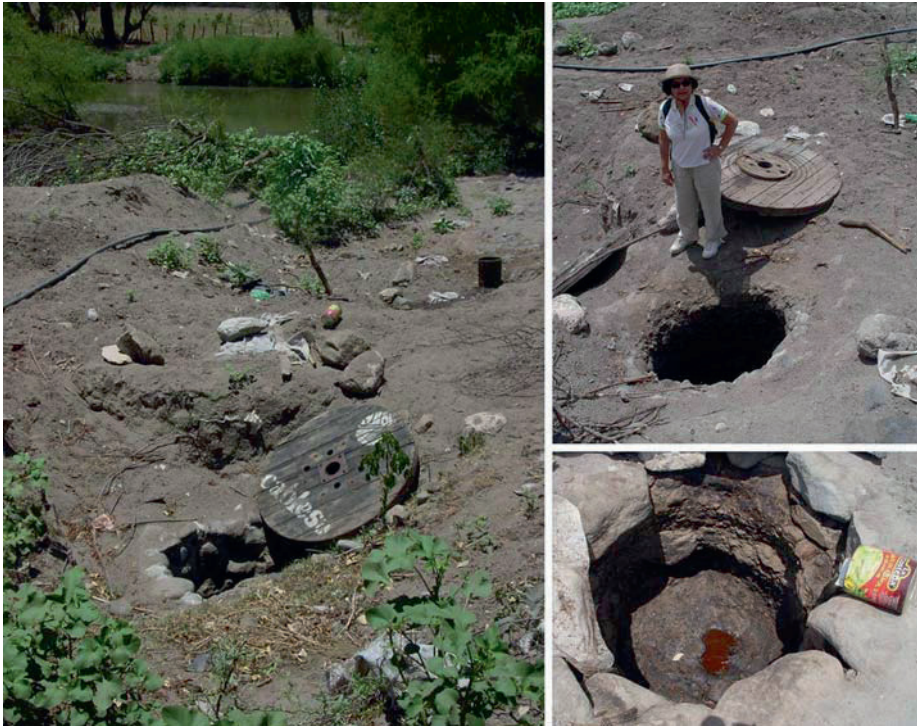
Fig. 5 Fermentation pits hand-hewn in the rock below ground level. Río Armeria. Canoas, Jalisco
