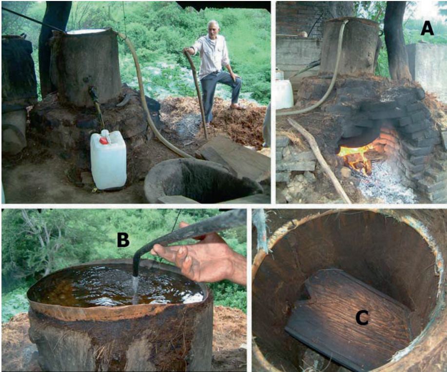
Fig. 6 A traditional “tavern”. Zapotitlán, Jalisco. (A) Filipino type still made out of a trunk of Enterolobium cyclocarpum (Jacq.) Griseb. The external receiver is an agave leaf. (B) Upper portion showing the condenser made with a copper pot and running water from the stream. (C) Inner receiver (“spoon”) made of wood
