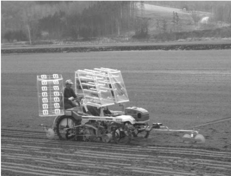
Fig. 9. A machine for transplanting onion seedlings.
