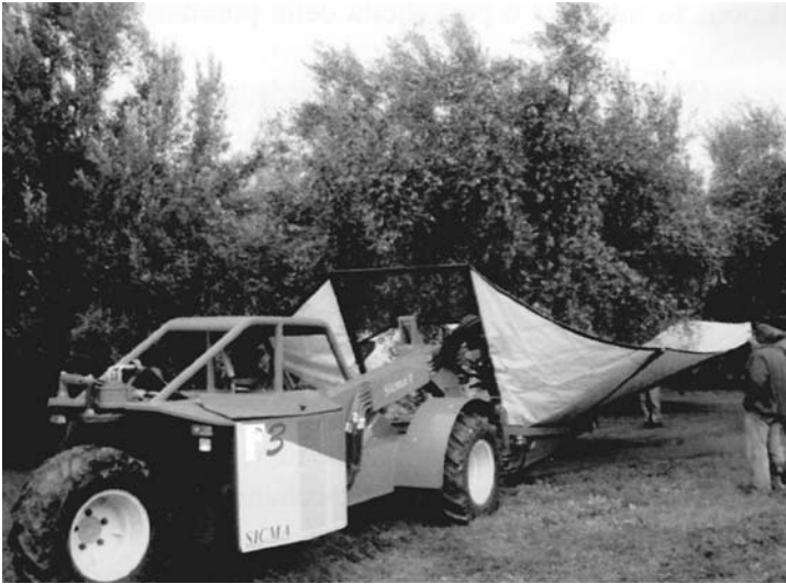
Fig. 22.2. Mechanical trunk vibrator with a reverse umbrella harvesting an olive tree (from Tombesi, 2006).
