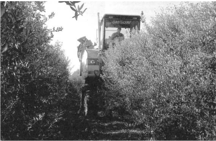
Fig. 22.4. An over-row olive harvester harvesting a super-high-density olive grove (from Tous et al. , 2006).
