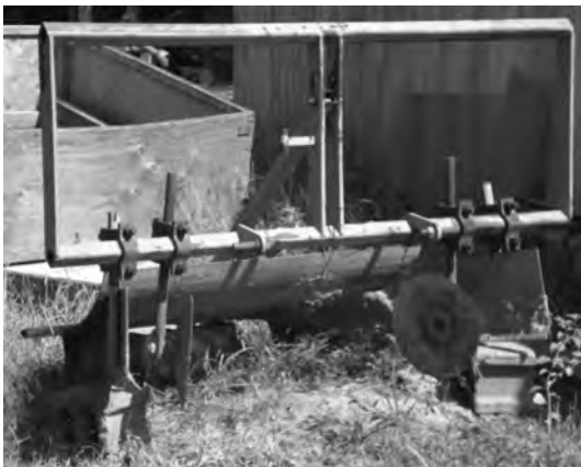
Fig. 7.5. A mechanical bed maker for pulling behind a tractor. The attachment makes beds 1 m wide and 20 cm high providing an elevated rooting environment for crops. Raised beds are often a sufficient remedy for minor drainage problems.
