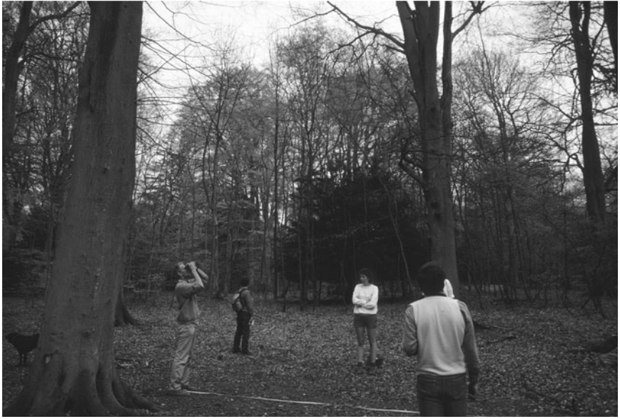
Fig. 3. 10 Measuring tree height using a hypsometer. The top of the tree is sighted through the instrument, and the distance from the tree is measured. Note that in deciduous forests, it is much easier to make measurements when the trees are leafless. (Photo by Adrian Newton.)
