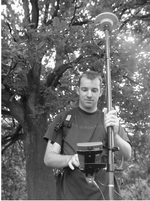
Fig. 3.3 A differential GPS system. The antenna and GPS receiver are illustrated here. A reference station is also required (not illustrated), which consists of an additional GPS receiver and antenna. Such systems can provide location data with an accuracy of a few centimetres. However, accurate measurements may be difficult to obtain under a forest canopy. This instrument is manufactured by Leica Geosystems AG of Switzerland. (Photo by Harry Manley.)
