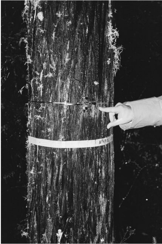
Fig. 4.11 Dendrometer band, affixed to a stem of the threatened conifer Fitzroya cupressoides . Dendrometer bands can be used to obtain very precise measurements of stem diameter increment in trees. (Photo by Cristian Echeverría.)
