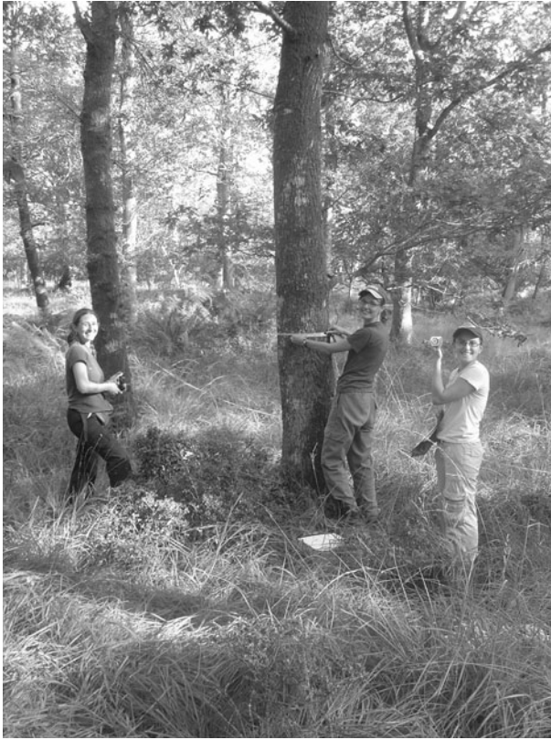
Fig. 3.9 Measuring stand structure in the New Forest National Park, southern England. The student in the centre is measuring diameter at breast height of an oak tree ( Quercus robur ) using a diameter tape. The others are carrying a laser rangefinder (left) and a hypsometer (right). (Photo by Adrian Newton.)
