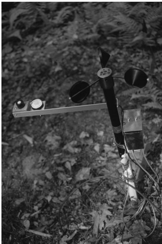
Fig. 4.9 A micrometeorological station for measuring light availability (using a PAR sensor) and wind speed (using an anemometer), to which a data-logger has been attached to record the measurements made. The instrument has been positioned in an experimental gap created at Harvard Forest, USA. (Photo by John Healey.)
