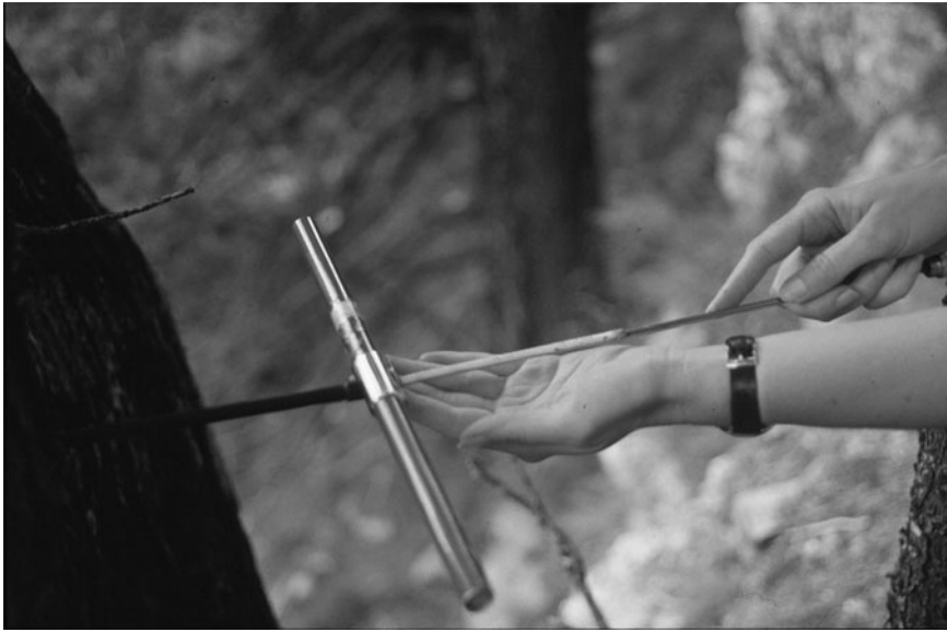
Fig. 3.8 Extracting the stem-core from an increment borer for dendrochronological analysis of growth rings. Great care is needed when extracting and transporting the cores, as they can be very fragile. (Photo by John Healey.)
