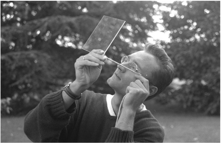
Fig. 4.8 The canopy-scope, a simple instrument that can be used for rapid assessment of forest understorey light environments (Brown et al. 2000). (Photo by Nick Brown.)
