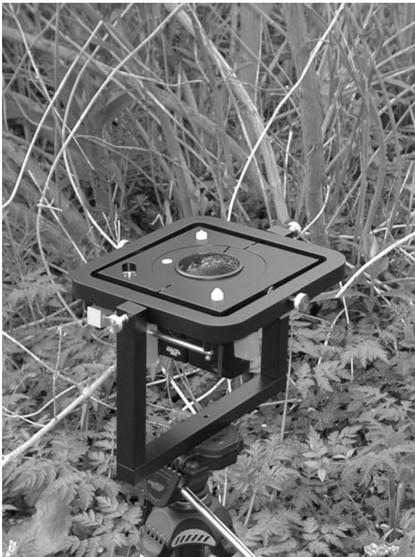
Fig. 4.4 The HemiView system used for taking hemispherical photographs of forest canopies. The system comprises a 180^\circ fisheye lens with a high resolution digital camera, mounted in a self-levelling camera mount to ensure that it is held horizontally. (Photo courtesy of Delta-T Devices Ltd.)
