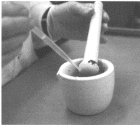
FIGURE 5.2 Sap extract is prepared by adding buffer to macerated leaf tissue and grinding.
