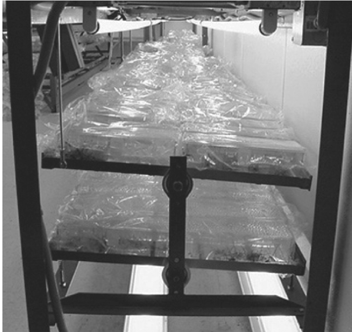
Figure 1. Agitated thin films are created by slowly pitching large rectangular vessels. Reproduced from Adelberg, J. (2004) [24] with permission from Society for In Vitro Biology.
