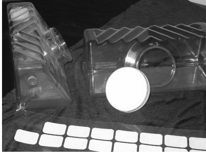
Figure 3. Liquid Lab Vessel ® for agitated thin film micropropagation with adhesive ventilation patches (shown in foreground).
