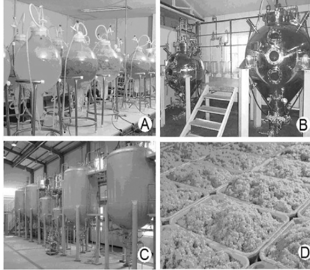
Figure 2. Scale-up of hairy-like adventitious roots of Panax ginseng . (A) 20-L balloon-type bubble bioreactors. (B) 500 and 1000-L pilot-scale balloon-type bubble bioreactors. (C) 10,000-L pilot-scale balloon-type bubble bioreactors for the commercial production of ginseng roots. (D) Harvested ginseng roots from a 10,000-L pilot-scale balloon-type bubble bioreactor. Photograph provided by Paek KY of CBN Biotech Co., Korea.
