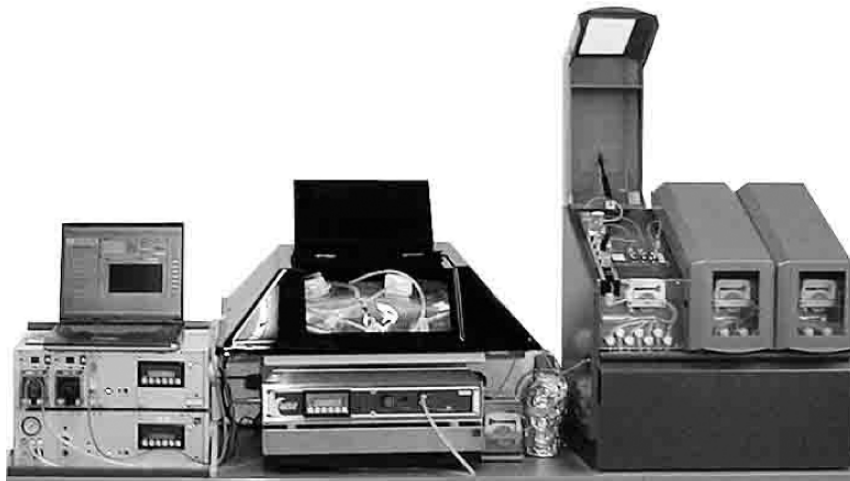
Figure 2. BioWave ® 20 SPS with ANTRIS for on-line measurement of metabolites.
