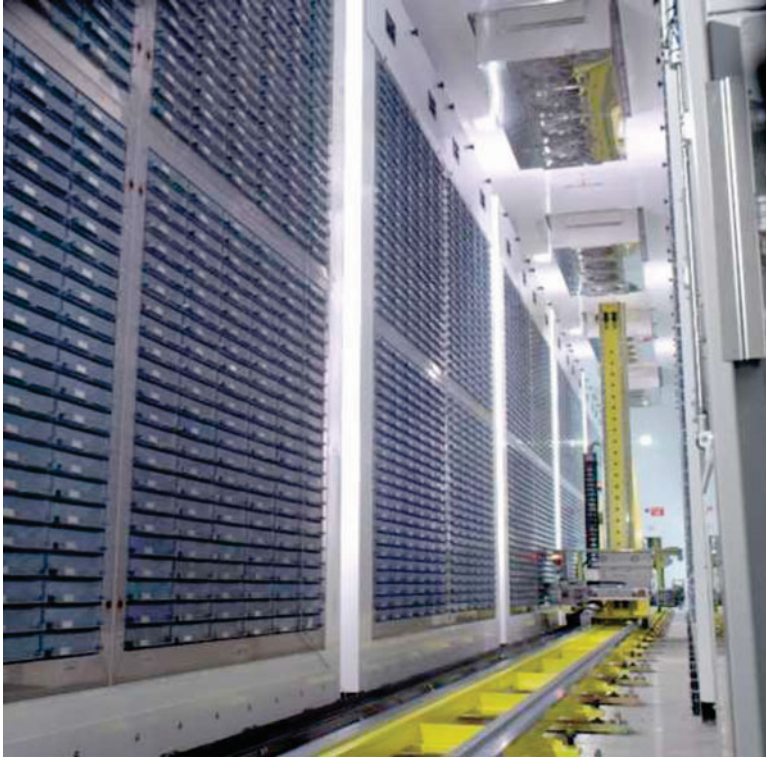
Fig. 2.2 Large automated -80^{\circ}\text{C} biorepository
