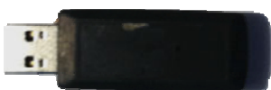
Fig. 3. A USB “keytyper” fob that, when inserted into a computer, will automatically launch Easy One Communicator in a kiosk mode
