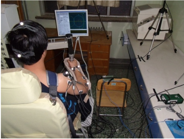
Fig. 2. Robot-aided movement data capture workstation
