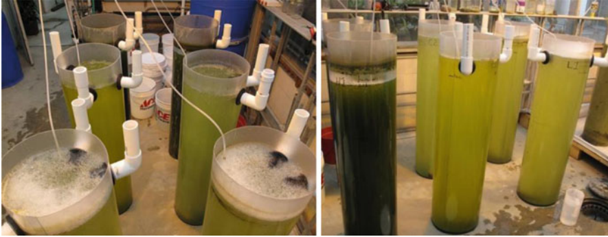
Figure 4. Monoculture and polyculture algae populations treating brewery wastewater (Sources: General Systems Research LLC & Dahiya et al., 2010).
