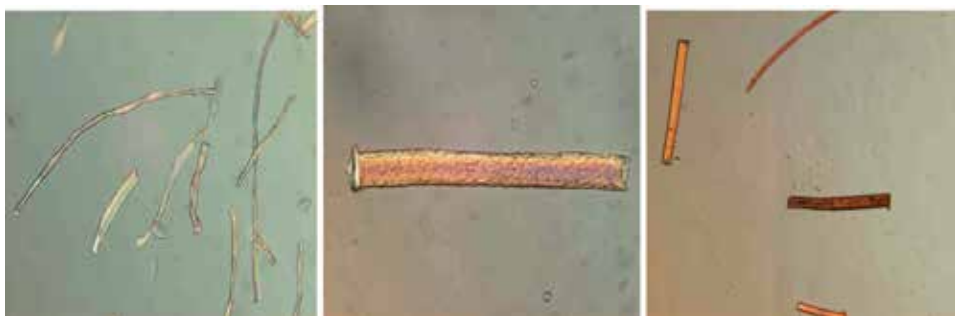
Figure 14. Cotton (left), true wool (middle) and colored (right) carpet wool fibers. University of Tabriz.
