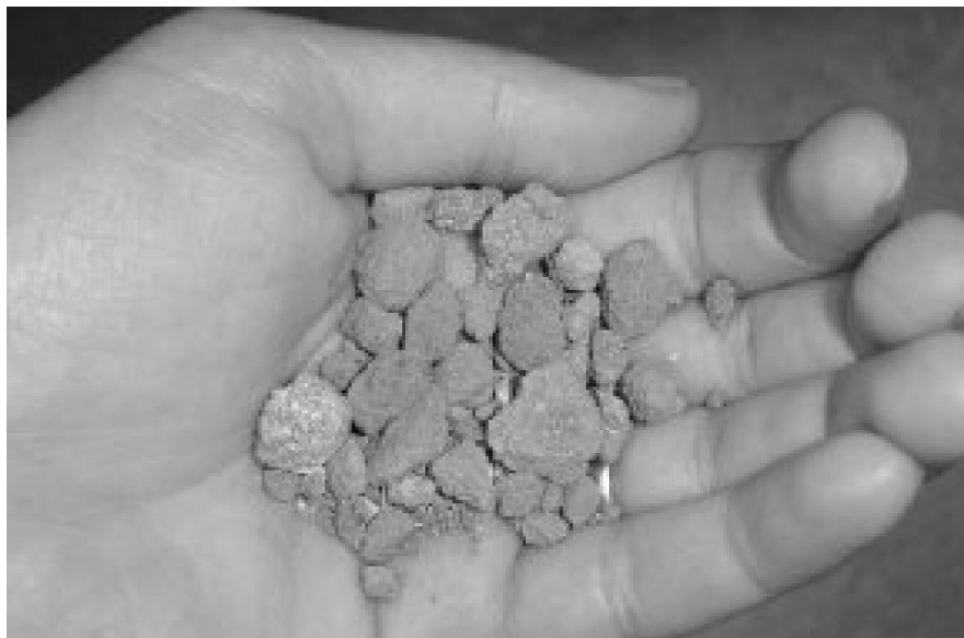
Fig. 4.1. Self-hardened and crushed wood ash. Photo: Anja Lomander.
