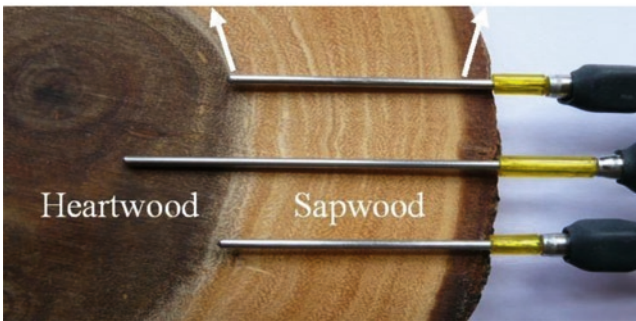
Fig. 4.3 Scheme of the measurement of sap flow density across stems using the multi-point sensors based on the heat field deformation method, HFD ( lower panel ). Sensors consisting of the heater ( middle needle ) and series of thermocouples (two needles symmetrically up and down the heater and one side needle, or two such needles – see Cermak et al. 2004) are installed in the sapwood along stem radius from different stem sides (e.g., cardinal points, up and down the slope, etc.) in order to cover natural variation. Typical results characterizes slightly asymmetric radial pattern of flow density related to root distribution ( upper panel ). Earlier studies confirm, that the flow in different sapwood layers near the stem base corresponds to water supply from roots growing in different depths – superficial and sinker. (Similarly it can be estimated flow into different crown parts, when sensors are situated at the crown base). Mathematical operations usually applied to separate poorly separated peaks allow separation of both fractions of flow (Nadezhdina et al. 2007; Cermak et al. 2008) roots are characterized according to their functions here. Superficial and sinker roots could have very different seasonal dynamics e.g., during drought
