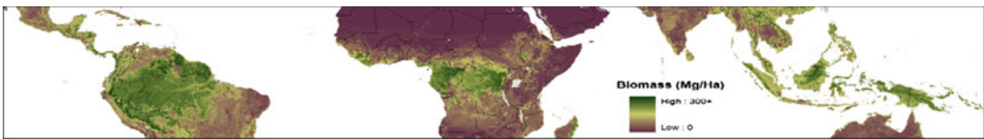
Fig. 9.2 The latest forest biomass carbon map for tropical forests has been developed by integrating optical (MODIS), lidar (GLAS), and RADAR (Alos) satellite data with field sampling. (Reprinted with permission)
