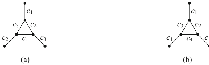
Fig. 1. (a) Edge-coloring using \chi'(G) = 3 colors, and (b) optimal edge-coloring using \chi'(G) + 1 = 4 colors, where \omega(c_1) = 1 and \omega(c_2) = \omega(c_3) = \omega(c_4) = 5
